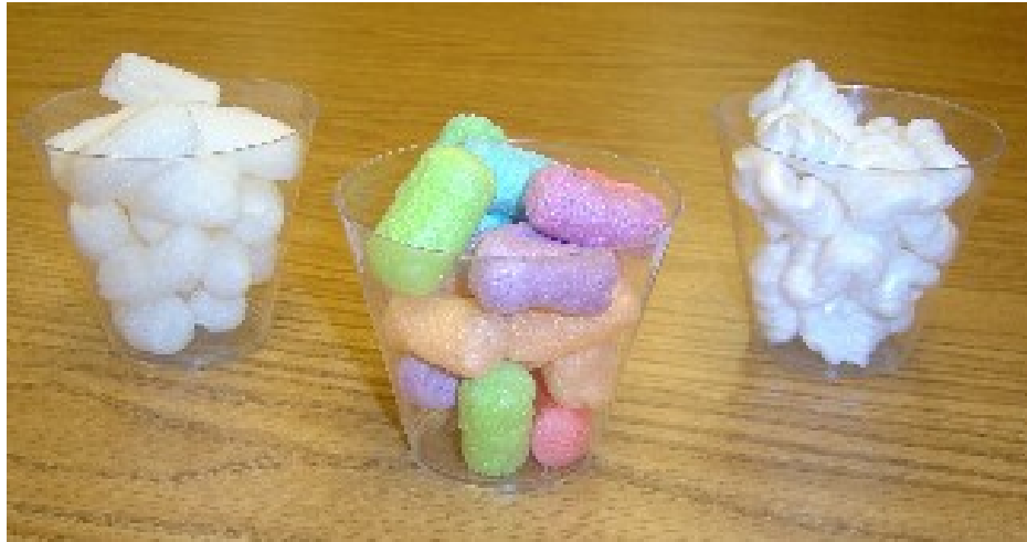
Figure 1. Cornstarch peanuts (left), dyed cornstarch peanuts (Magic Noodles - middle), and Styrofoam peanuts (right).
