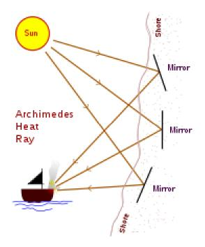
**Caption (b):** A possible array of mirrors used to set fire to enemy ships with Archimedes' weapon. **Source:** https://en.wikipedia.org/wiki/Archimedes
