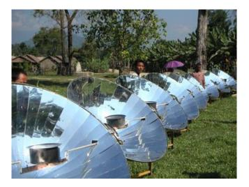
**Caption (c):** Examples of parabolic mirrors used for cooking. **Source:** https://science.howstuffworks.com/environmental/green-science/solar-cooking.htm
