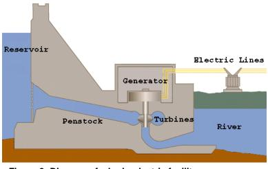
Figure 2: Diagram of a hydroelectric facility
